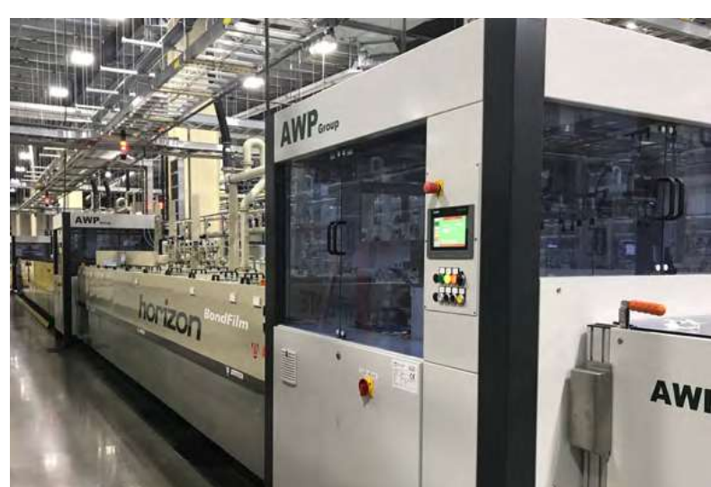
Figure 2: BondFilm LDD SR (splash reduction on laser-drilled holes followed by desmear processing).
